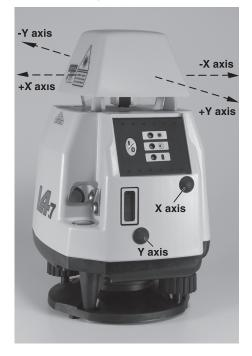
**3.** Center the circular level vial and turn the laser on.
