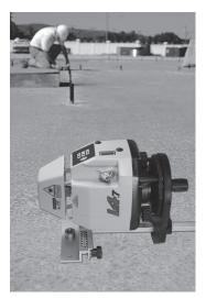
Along with the ability to project a level reference plane, both **L4.7** models have a built-in, manually leveled vial, for aligning the plane of light vertically. The optional W1 mount is used for this application.
