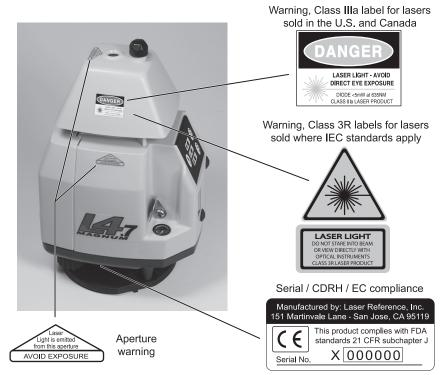
**Note:** The **L4.7 MAGNUM** transmitter is a class 3R laser under the 1993 IEC 825-1 laser safety standard and revised edition of EN60825. The **L4.7 MAGNUM** laser conforms to applicable EC directives regarding RFI and EMI.
